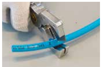
Correct tube cut with metal tube cutter
