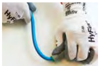
Fitting with tube inserted, having a tight bending radius
