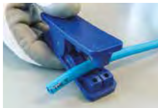
Tube cut at 90° with plastic tube cutter
